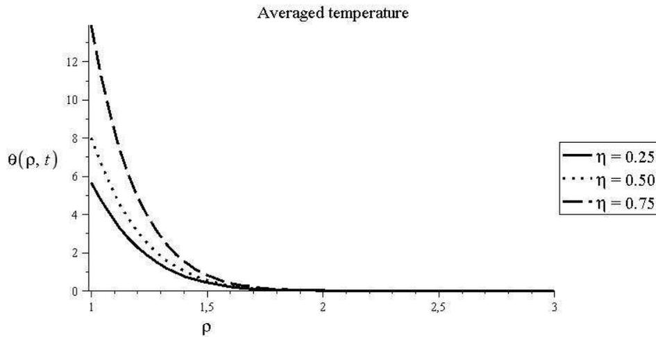
Fig. 5. Fibres width effect on averaged temperature after one hour
