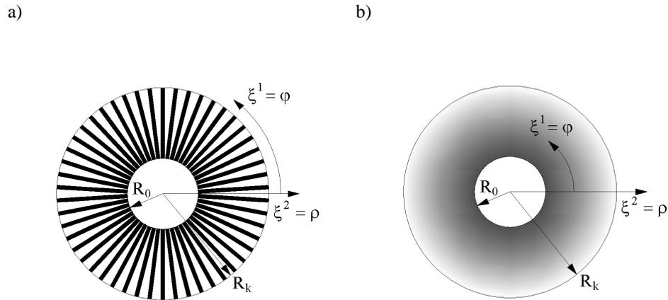
Fig. 1. Structure of the two-phase functionally graded composite in a) micro- and b) macro-scale
