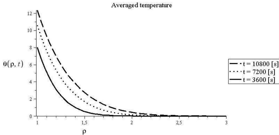
Fig. 4. Averaged temperature varying in time
